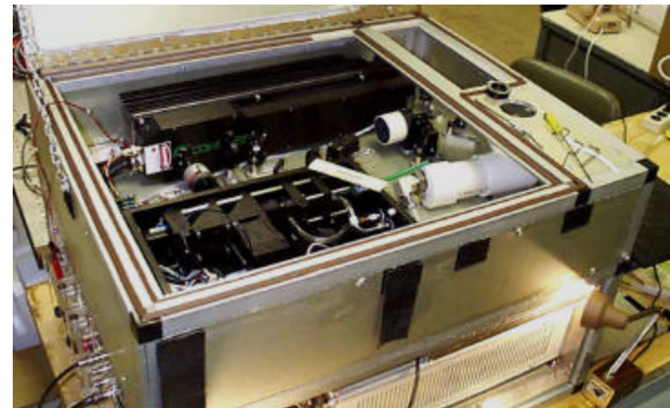
Current Instrument with COTS Nd:YAG laser (4"x4"x16" and 6"x19"x18")
